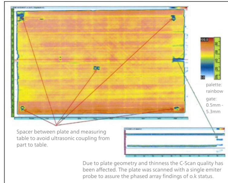
Figure 4 (a). C-scan chart for oven consolidated laminate
