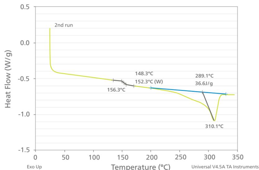
Figure 1 (c). Second run DSC on raw polymer
