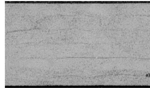
Figure 5a. Polished optical micro-sections of unidirectional laminate consolidated out of autoclave.
