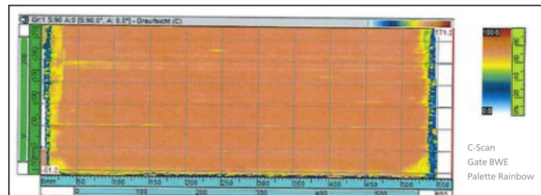
Figure 3. C-scan of AFP laid laminate consolidated in a press
