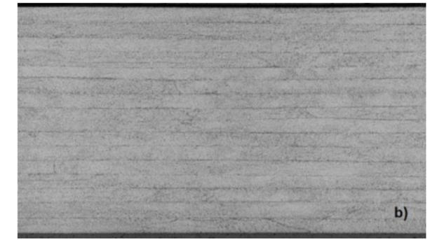
Figure 5b. Polished optical micro-sections of ± 45 laminate consolidated out of autoclave.
