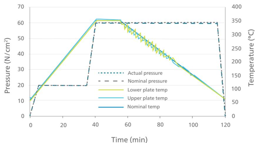
Figure 2. Press cycle for tapes laid by automated fibre placement (AFP)
