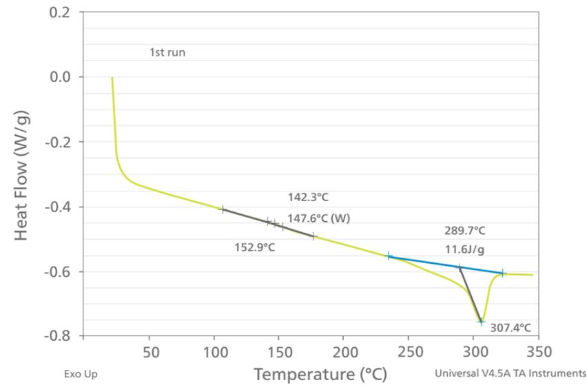
Figure 7. Example DSC thermograph for platen pressed laminate.
