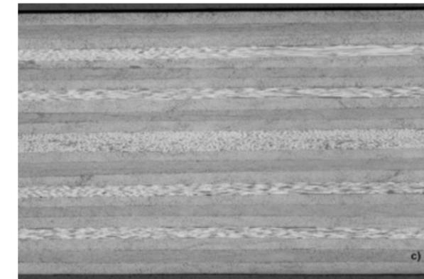
Figure 5c. Polished optical micro-sections of quasi-isotropic laminate consolidated out of autoclave.
