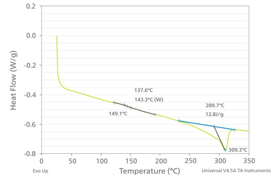
Figure 6. Example DSC thermograph for oven processed laminate
