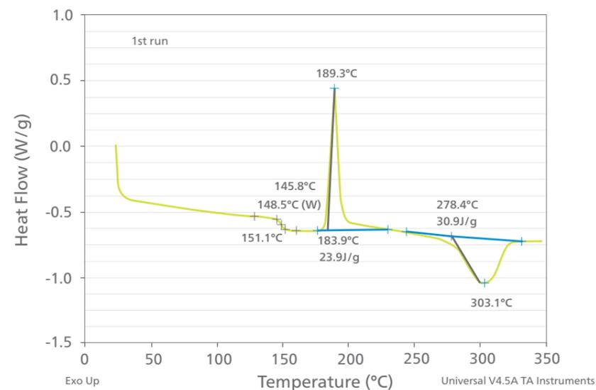
Figure 1 (a). First run DSC on raw polymer
