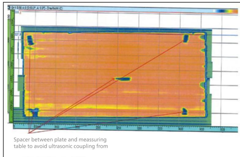
Figure 4 (b). C-scan chart for press consolidated laminate
