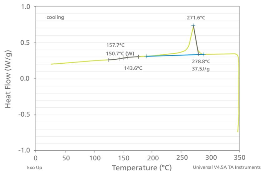
Figure 1 (b). Cooling curve DSC on raw polymer
