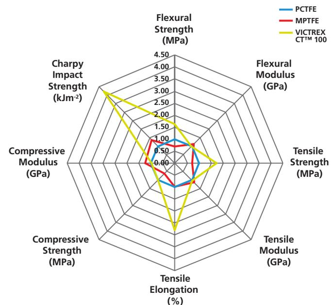
It is evident that there is a greater change in the properties of the fluoropolymers from ambient to 77K than for VICTREX CT™ 100 polymer: the latter material exhibits more than three times higher impact strength and elongation at break than the fluoropolymers while maintaining higher strength.
