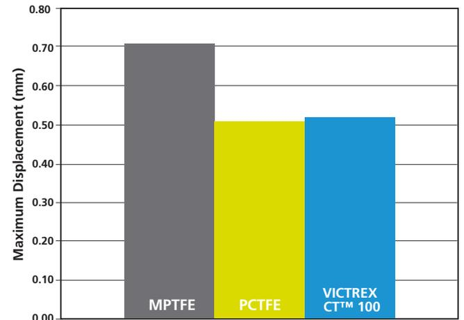
Figure 9: Residual Displacement on removal of load from seat
