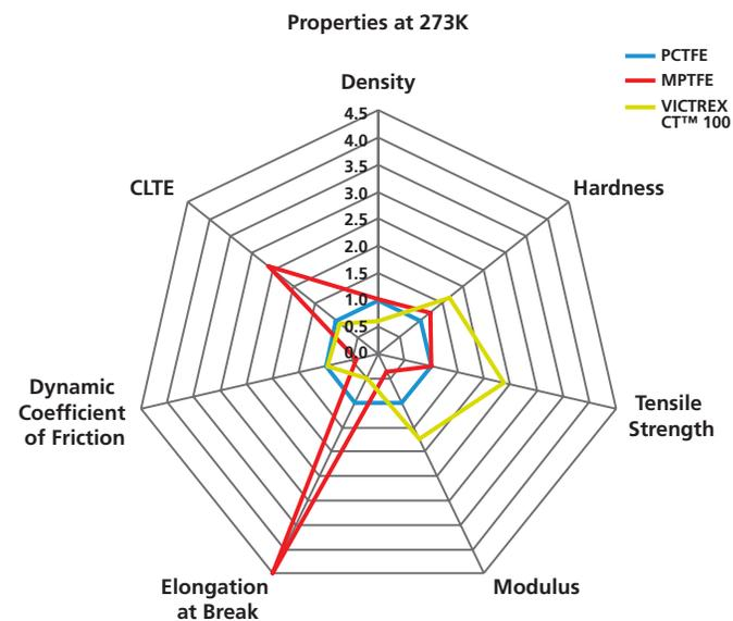
The simple star chart shows VICTREX CT™ 100 polymer with a significantly higher tensile strength and modulus than PCTFE and MPTFE, higher hardness and a lower elongation at break. Dynamic coefficient of friction is similar while thermal expansion coefficient is significantly lower. Notably the density of VICTREX CT™ 100 polymer is some 40% lower than the fluoropolymers.
