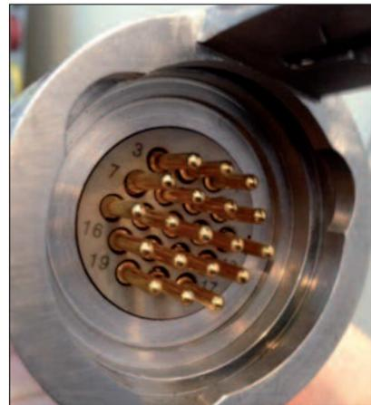
Figure 4. In electrical connectors for down-hole and subsea environments VICTREX PEEK often replaces glass, ceramic and thermosetting resins because of its high mechanical strength and creep resistance at temperature. In addition, the material has the ability to act as an inherent seal at pressure differentials up to 345 MPa (50 000 psi) in a variety of corrosive environments, including hydrogen sulfide (sour gas) and sea water.
