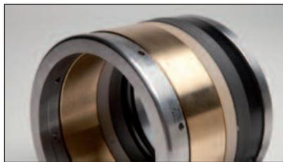
Figure 3. CDI plunger packing is traditionally a multi-material stacking assembly, comprising seal rings made of polytetrafluoroethylene, VICTREX PEEK, rubber and steel. The packing is typically used in positive displacement pumps rated up to 138 MPa (20 000 psi).
