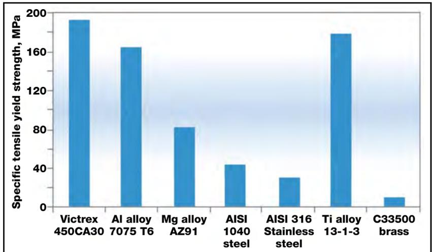
Fig. 1 — PEEK polymers provide equivalent stiffness at lighter weights.
