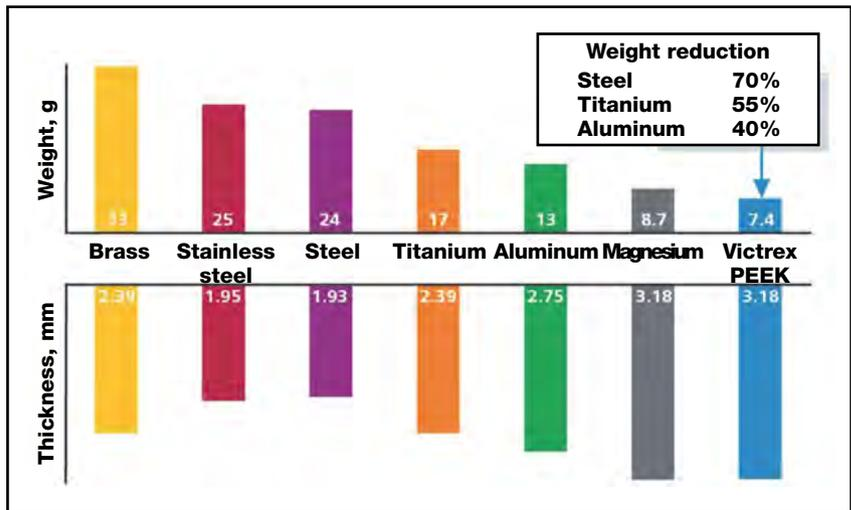
Fig. 2 — Parts made of PEEK polymers weigh less than metal counterparts, but have higher specific strength.
