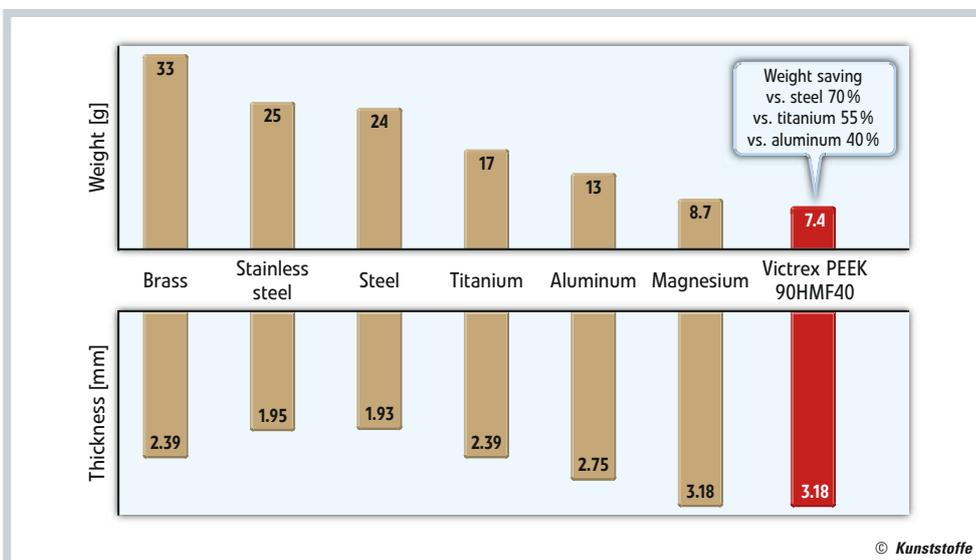
**Fig. 5. Reinforced with carbon fibers, Victrex PEEK HMF enables significant weight reduction as against metals: A comparison of different material specimens of the same rigidity, concerning thickness and weight** (figure: Victrex)
