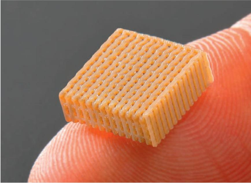
**Fig. 1.** Fine detailed porous structure printed in Victrex PEEK using Bond3D technology (© Bond High Performance 3D Technology)
