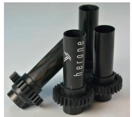
**Fig. 3.** Drive-shaft system consisting of a braided preform made of Victrex AE250 thermoplastic UD tapes overmolded with an integral gear made of Victrex PEEK 90HMF40 (© herone)
