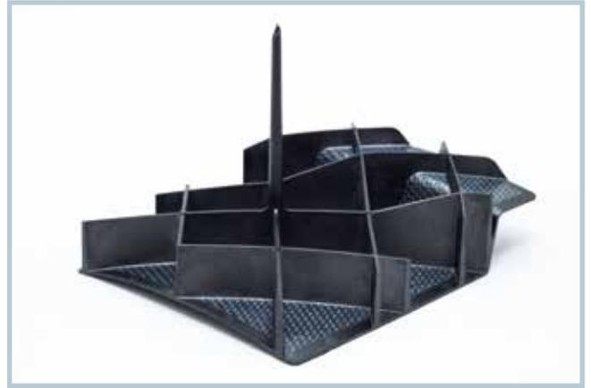
**Fig. 2.** Combines high strength and light weight: Grid stiffened demonstration panel, a Victrex PAEK thermoplastic composite overmolded with Victrex PEEK (© TPRC)
