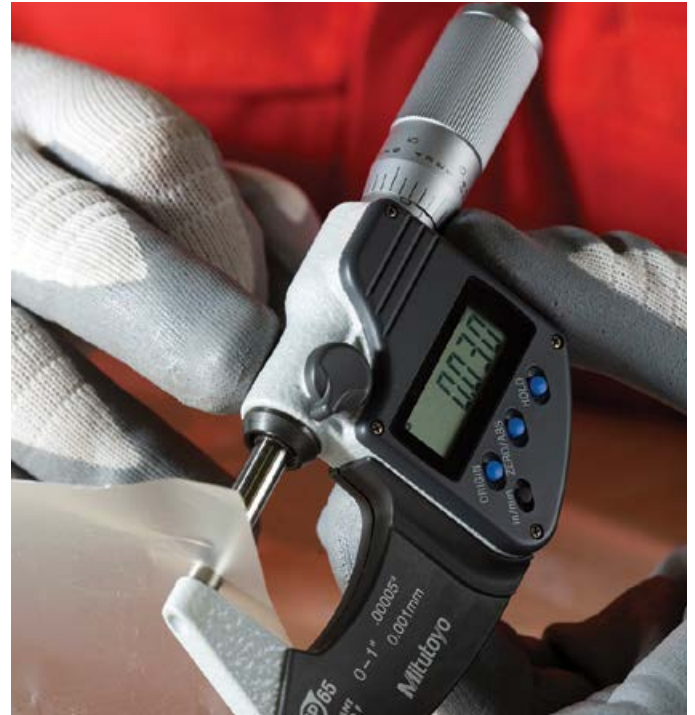
Measuring the thickness of extruded APTIV Film.
