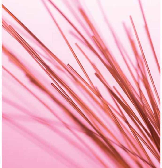
Extruded VICTREX PEEK fibres.
