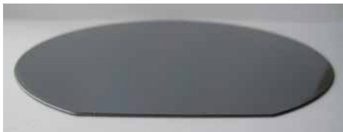
Figure 3 1 : BOPEEK film laminated on a silicon carrier
