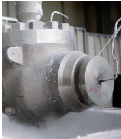
Figure 9. 10 inch diameter trunnion ball valve test
