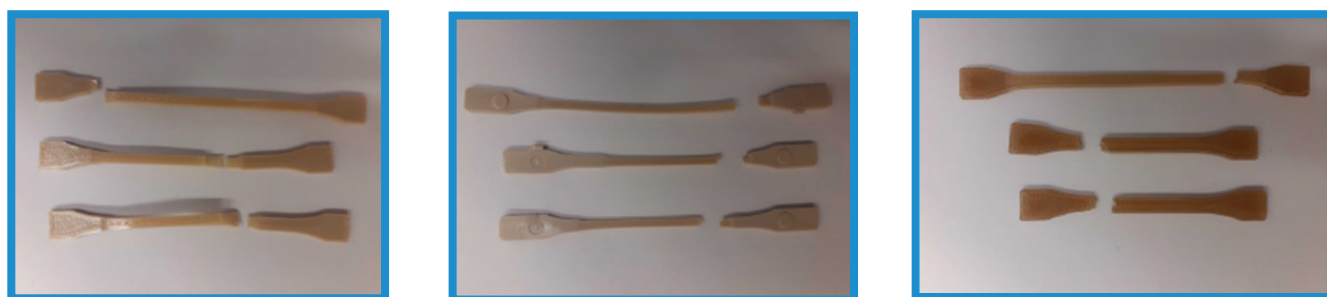
Figure 1. ISO527-2-1BA bars in Injection moulded LMPAEK (left), VICTREX AM™ 200 printed crystalline (centre) and printed amorphous (right)
