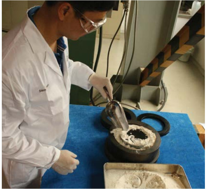
Clean tools must be carefully filled with the correct amount of VICTREX PEEK powder.
