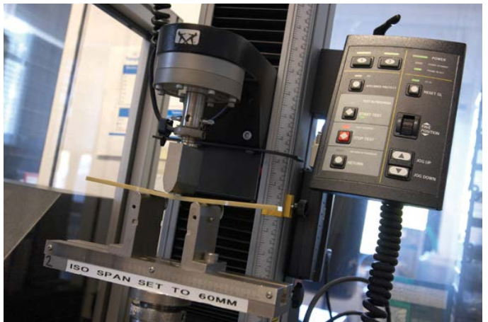
Flexural testing may be carried out to monitor the quality of compression moulded parts.
