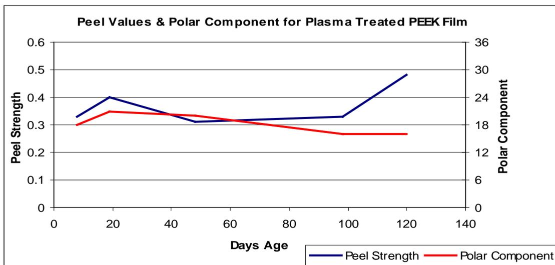
**Figure 2 – Peel Strength (N mm<sup>-1</sup>) and Polar Component (mJ m<sup>-2</sup>) Ageing Over 120 Day Time Period**
