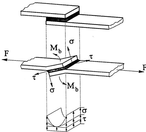
The upper picture shows two specimens which are bonded with an overlap. Applying a force  $F$  on either end of the shear joint will bend the sample as shown in the central part of the figure. Bending occurs since the point of application of  $F$  is not in line with the joint. Therefore we find a bending moment  $M_b$  leading to a tensile stress  $\sigma$ . The tensile stress by itself may be viewed as acting like a peel stress.
