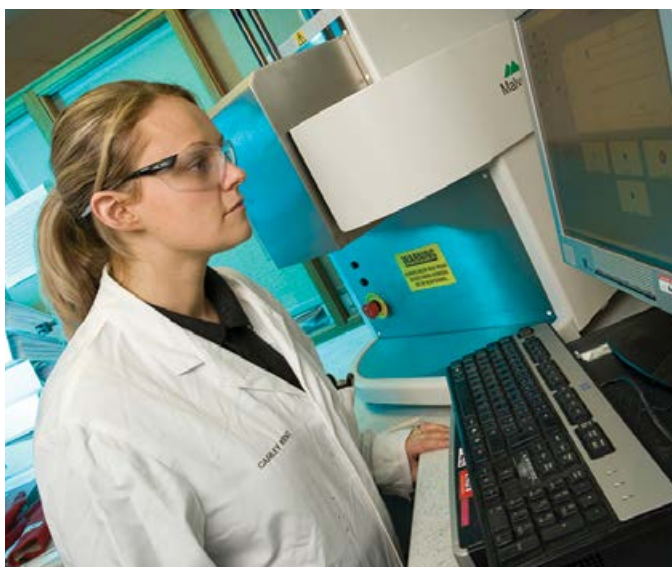
State of the art test equipment is used to measure shear viscosities.
