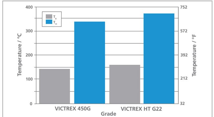
The molecular structure and semi-crystalline nature of VICTREX HT results in a melting point (T<sub>m</sub>) 30°C (54°F) higher and a glass transition temperature (T<sub>g</sub>) 14°C (25°F) higher than VICTREX 450G.
