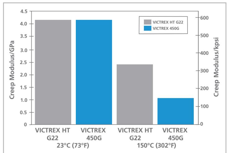
While the creep modulus of VICTREX HT and VICTREX 450G are very similar at room temperature, VICTREX HT has a creep modulus more than twice that of VICTREX 450G at 150°C (302°F). This means that VICTREX HT can support higher loads than VICTREX 450G at 150°C (302°F) without permanent deformation.
