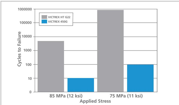
The molecular structure and semi-crystalline nature of VICTREX HT results in much better resistance to fatigue than VICTREX 450G at high levels of stress.
