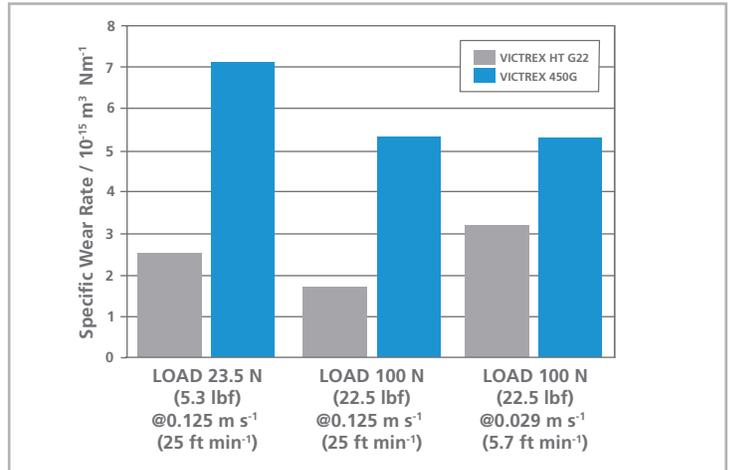
In thrust washer tests performed under different PV conditions, VICTREX HT exhibited as little as 1/3 the wear of VICTREX 450G. VICTREX HT showed a lower specific wear rate than VICTREX 450G under all other test conditions.
