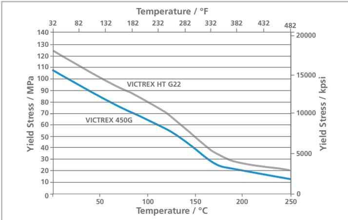
The temperature resistance of VICTREX HT allows it to be used an average of 25°C (45°F) higher temperatures than VICTREX 450G.
