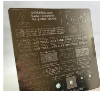
VICTREX™ PEEK plaque metallised via Surface Activation™ technology
