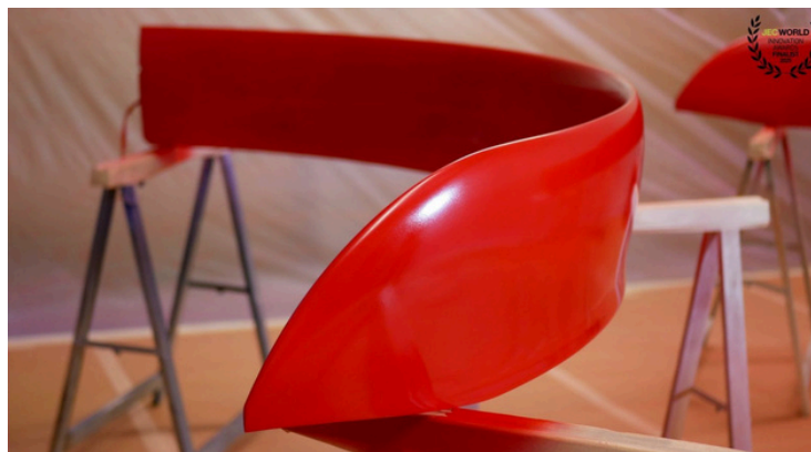
Completed LMPAEK™ thermoplastic Hydrofoil by Minilab
