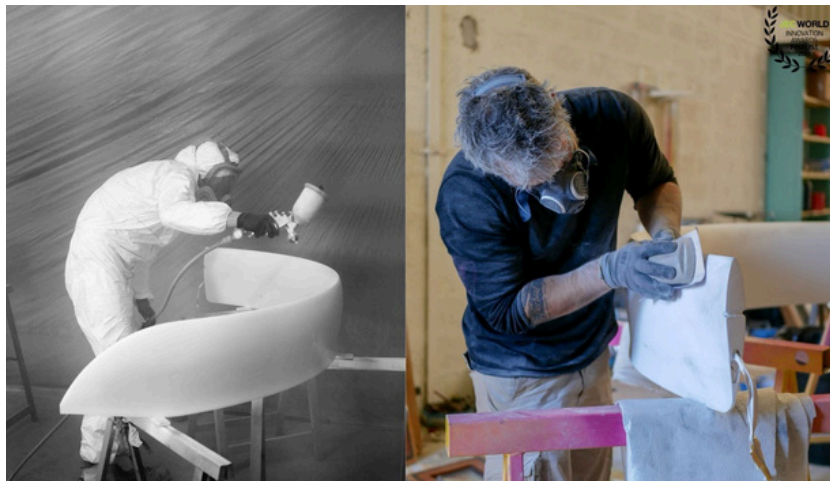
Hydrofoil manufacturing steps : (polishing and painting)
