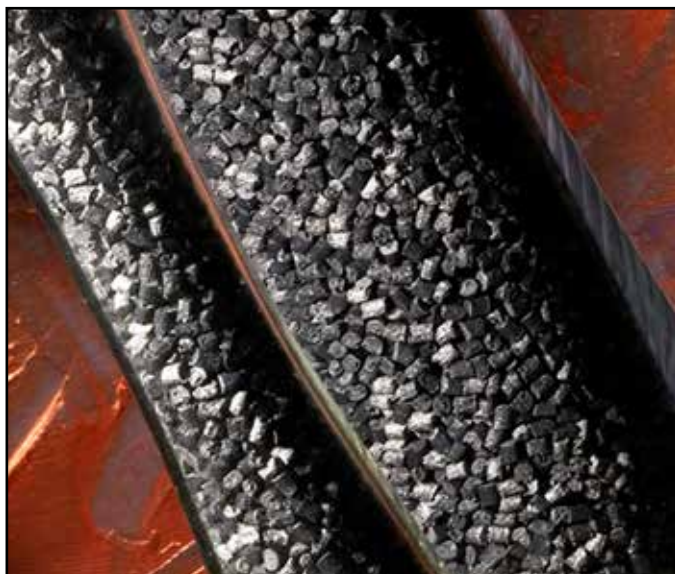
Figure 3: Short carbon fiber injection molded VICTREX PEEK polymer
