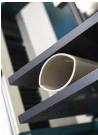
Crush resistance testing used to measure robustness of the pipe.
